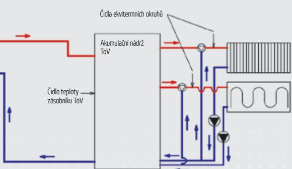
ZAPOJENÍ FRESH STANICE SE SYSTÉMEM TEPELNÉHO ČERPADLA
