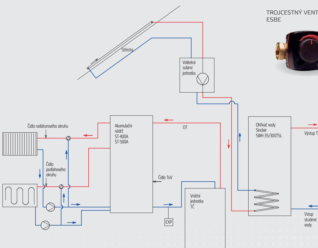
V TOMTO ZAPOJENÍ LZE POUŽÍT REŽIM CHLAZENÍ LIBOVOLNÝMI FANCOILY
